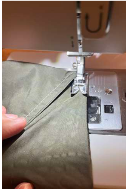
each cut on the ripstop nylon is french seamed to have it hold the puff shape once sewn to the elastic
