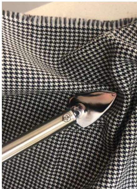
molded leather with baby iron. pressed parts of it onto fabric with double glue or on fusing itself if lined
